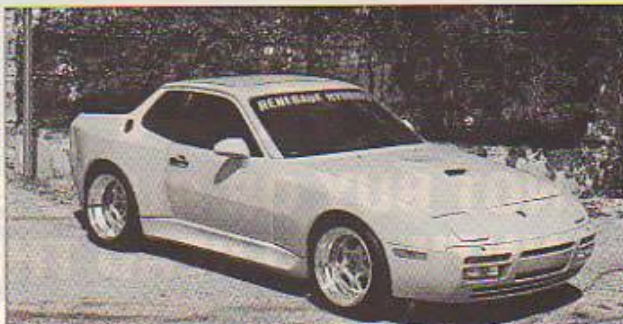
The exaggerated fender flares of IFC's Wide Body create a more menacing look for either a 924 or 944 Porsche.
